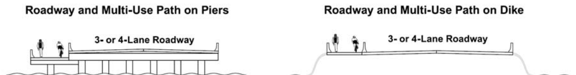
Figure 9: OR 126W Causeway Design Options
