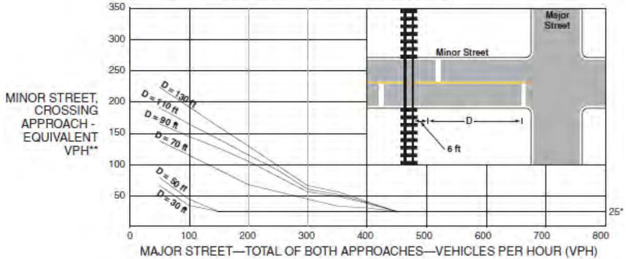
Figure 4C-9. Warrant 9, Intersection Near a Grade Crossing (One Approach Lane at the Track Crossing)
